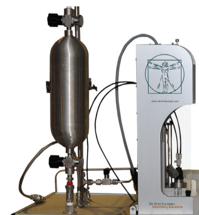
Figure 3. GDI transformed to a GC injector
