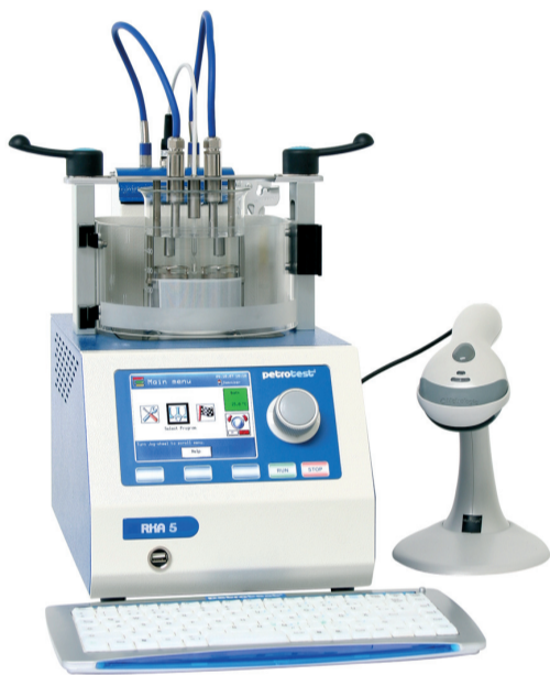
Fig. 1: The RKA-5 automated ring and ball tester
