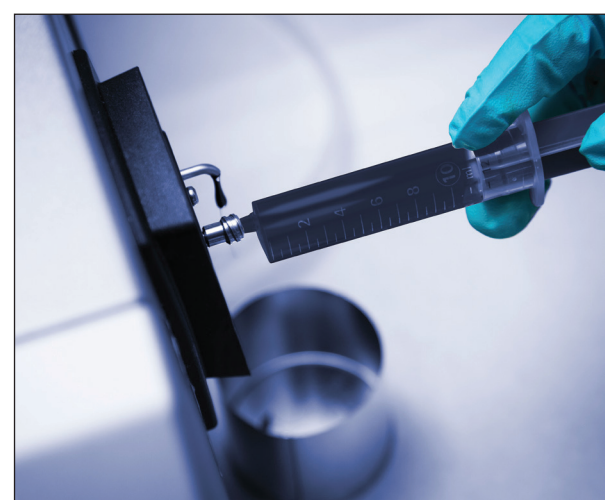
Figure 1. A hot bitumen sample is injected into the heated DMA 4200 M measuring cell
