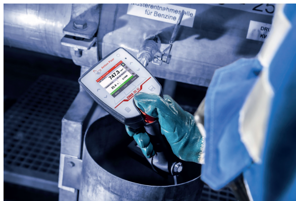
Figure 5: Intrinsically safe DMA 35 Ex Petrol in use in hazardous area
