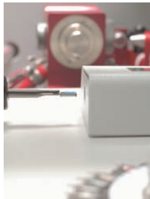
Figure 2: The autosampler SSA 600 carries solid samples on a graphite platform directly into the graphite furnace.
