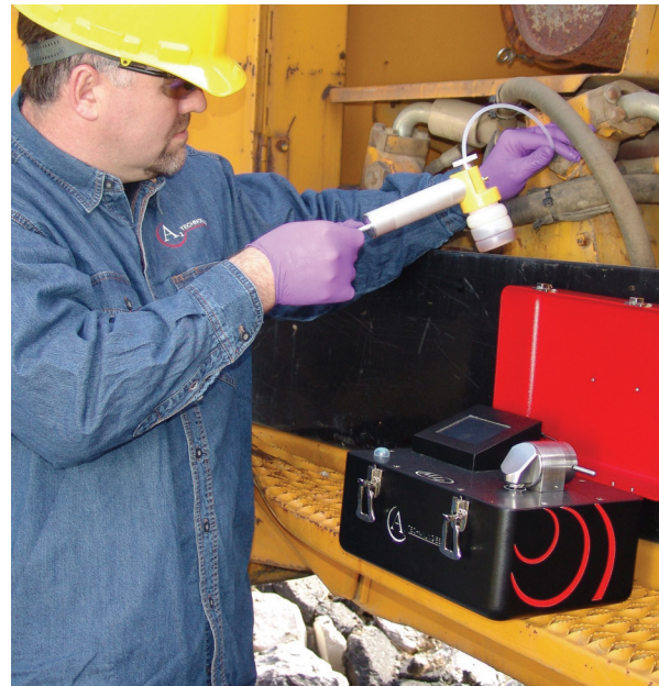
Lubrication sample is drawn for at site analysis by A2 Technologies Mobility FTIR Spectrometer
